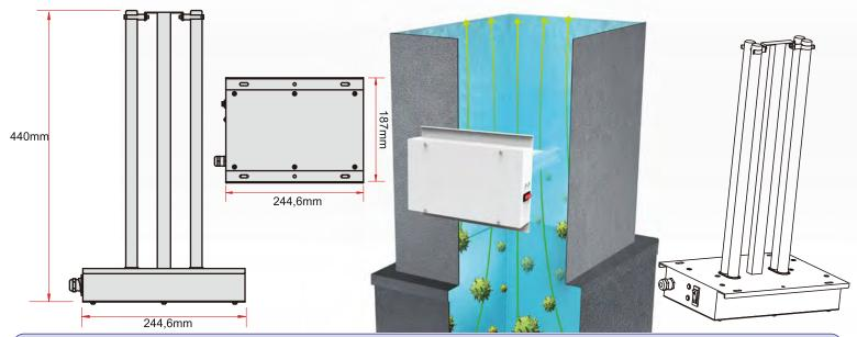
72-watt UV-C germicidal lamp, suitable for air sterilization in ducts of hospitals, gyms, schools, restaurants, apartments, shops, offices. Made of AISI 304 stainless steel. It has a lamp life greater than 8000 hours. Net weight of Kg. 1,1. Inserted inside the air conditioning ducts, it eliminates the bacterial load.
