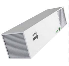
Appliance model NLUVAIRCOND36 **Emitter power** 36W UV wavelength UV-C 253.7nm Nominal capacity of treated air 5.6 m<sup>3</sup> per minute Irradiation µw / cm<sup>2</sup>  $\geq$ 110µw / cm<sup>2</sup> Treated area per room H 3mt. and three air changes per hour 36 m2
