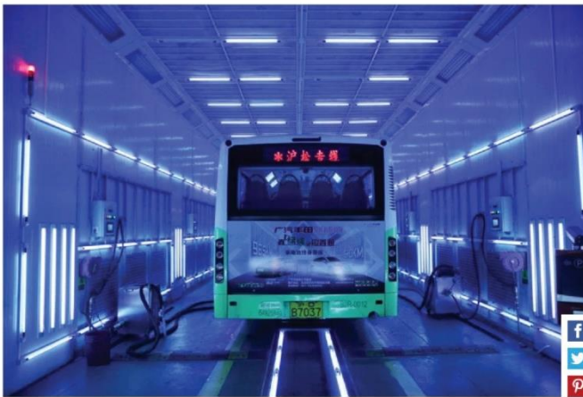
A bus is disinfected by ultraviolet light (Picture: China News Service via Getty Images)
